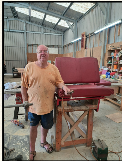
Three of our seat frames for A1477 had to be modified to suit the seat backs. Richard Ellis here with a successful result. Richard Stratford did the welding and grinding.
